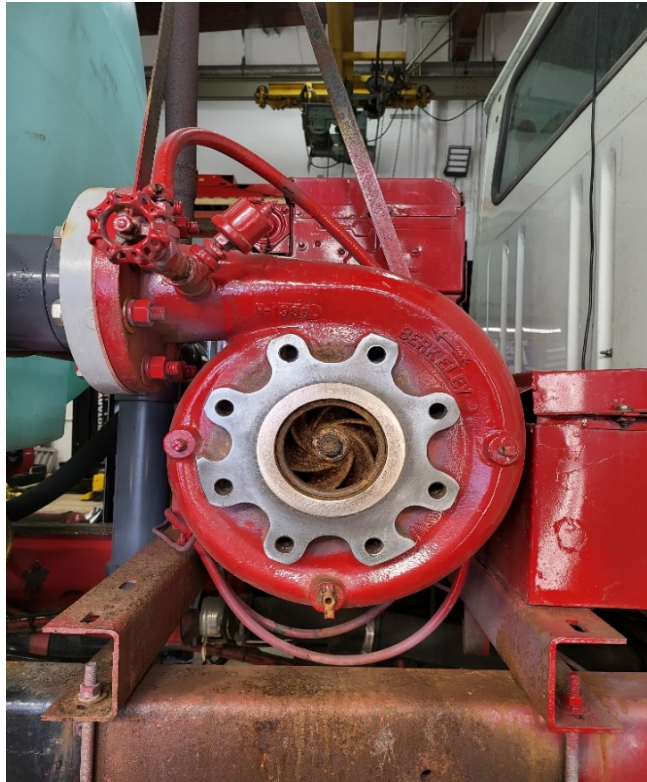
Flush Truck Pump Rebuild
